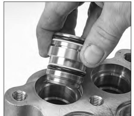
1.47 The V-packing spacer has two distinct steps. Press the longer side with the groove into the inlet manifold.
