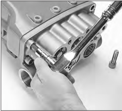
1.09 Use a 10 mm hex socket to remove the four (4) HSH screws from the inlet manifold.
