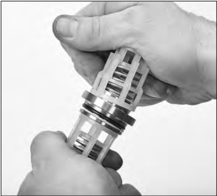
2.35 Push assembly together until it snaps into place.
