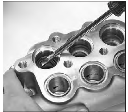
1.14 Repeat for the second V-packing, inspect both for wear or damage.
