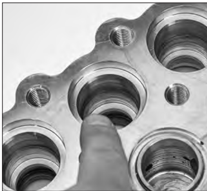
1.16 Inspect the manifold bore to ensure sealing surface is smooth and free from corrosion.
