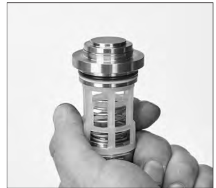
2.32 Place discharge valve onto discharge valve seat with tapered surface facing down.
