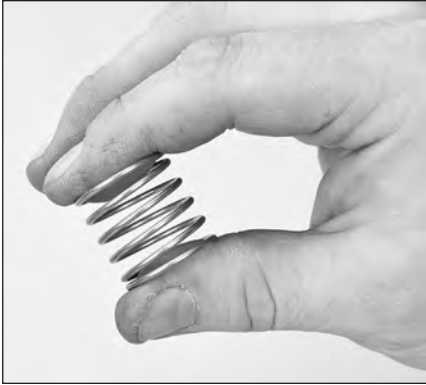
2.20 Inspect spring for proper tension or any damage.
