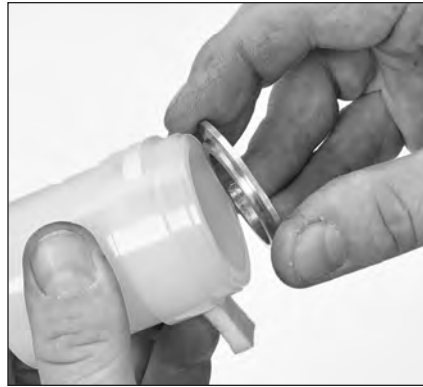
1.21 Remove low-pressure seal washer.
