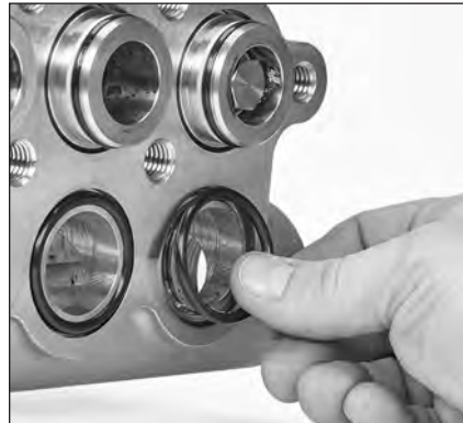
1.52 Replace inlet manifold O-rings.
