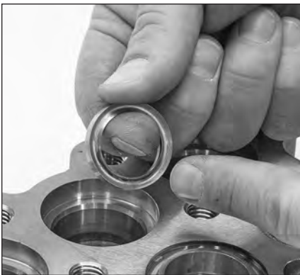
1.15 Remove the female adapter and inspect for wear or damage.
