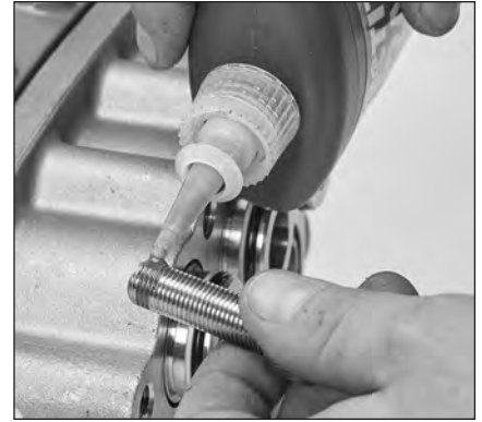
1.50 Place a drop of Loctite® 242® on the threaded end of the four (4) HSH screws and install by hand.
