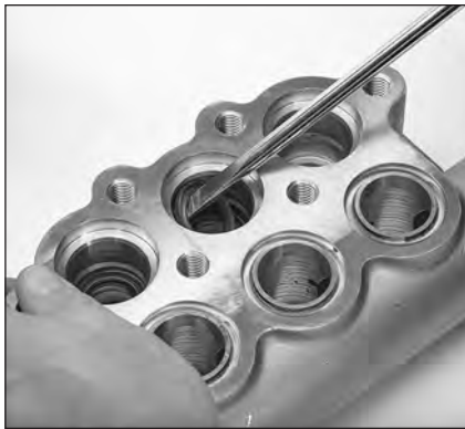
1.13 Use a flat tip screwdriver to pry the first V-packing upward and remove.
