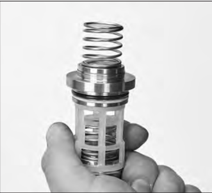
2.33 Place spring onto stepped side of discharge valve.
