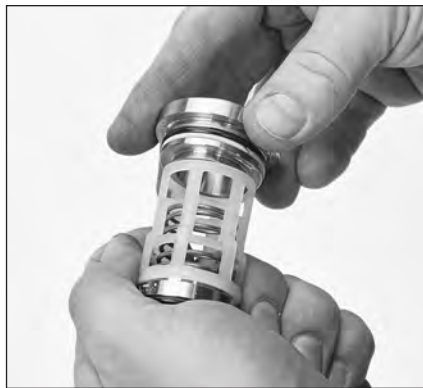
2.31 Install discharge valve seat onto inlet spring retainer and push assembly together until it snaps into place.
