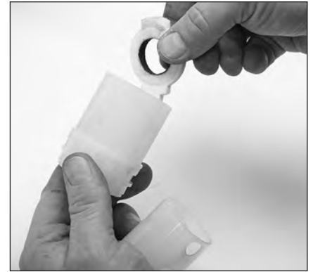
1.22 Seal retainer can be separated to remove and inspect the wicks. Replace as needed (wicks not included in the seal kit).
