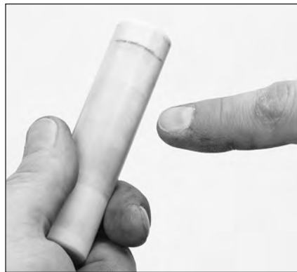
1.27 Inspect ceramic plunger for cracks and scoring to the surface. Clean with a wire-wheel brush if necessary.
