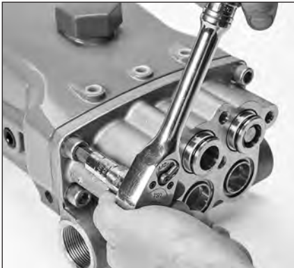
1.51 Using a 10 mm hex socket, tighten HSH screws. Torque to 355 in-lbs, 30 ft-lbs, or 40 Nm.
