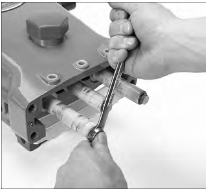
1.23 Using a 14 mm combination wrench, loosen the plunger retainer.
