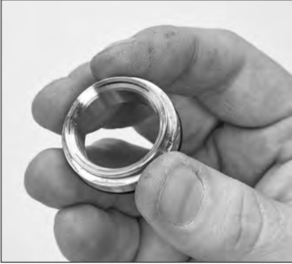
2.22 Inspect tapered surface of inlet valve seat for wear, pitting or damage.
