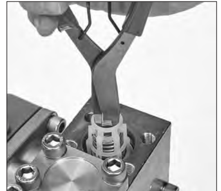
2.06 Use a reverse pliers to grasp the center of the valve spring retainer. Twist while pulling away from manifold to remove valve assembly.
