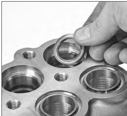
1.42 The female adapter has a flat side and a grooved side. Install with the groove side facing up.
