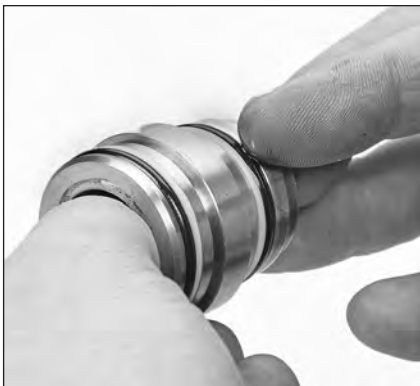
1.46 Apply a lubricant to the V-packing spacer O-rings.
