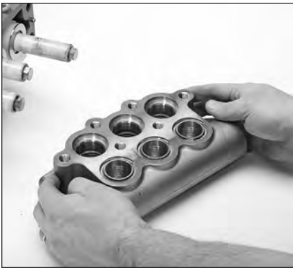
1.12 Remove inlet manifold by hand and place on a flat surface with V-packing spacer bores facing up.
