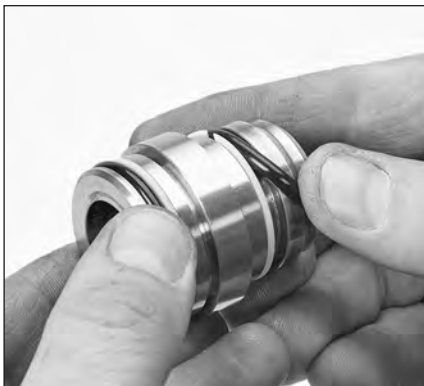
1.45 Install backup rings, then O-rings onto the V-packing spacers.
