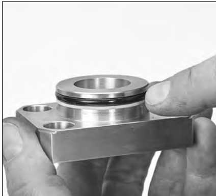
2.04 Inspect valve plug O-ring and backup ring for cuts, nicks or damage.
