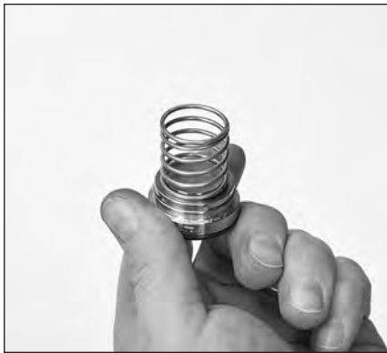
2.27 Place spring onto stepped side of inlet valve.
