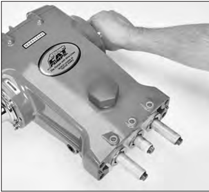
1.48 Rotate crankshaft so outside two plungers are even at furthest distance from crankcase.
