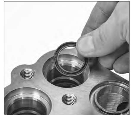
1.44 Install the second V-packing with the groove side also facing up.
