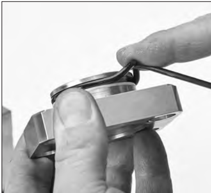
2.05 Using a pick, remove O-ring and backup ring from valve plug.
