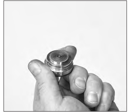
2.26 Place inlet valve onto inlet valve seat with tapered surface facing down.
