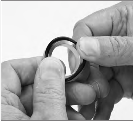
2.24 Replace inlet valve O-ring.
