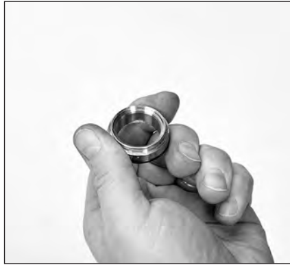
2.25 Hold inlet valve seat with tapered surface facing up.
