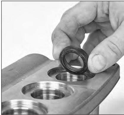
1.40 One side of the low-pressure seal has a groove. Install groove side facing down and press into place.
