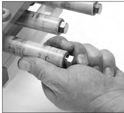
1.24 Before completely removing the plunger retainer, stop and push the plunger towards the drive end to break loose from the retainer. Remove the plunger and retainer.
