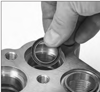
1.43 Install the first V-packing with the groove side facing up.
