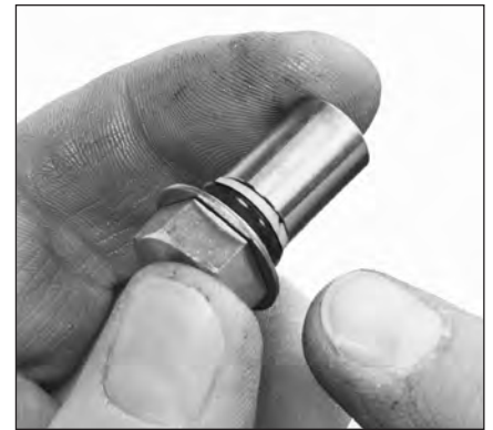
1.25 Remove the plunger retainer from the plunger and inspect the O-ring and backup ring for damage.
