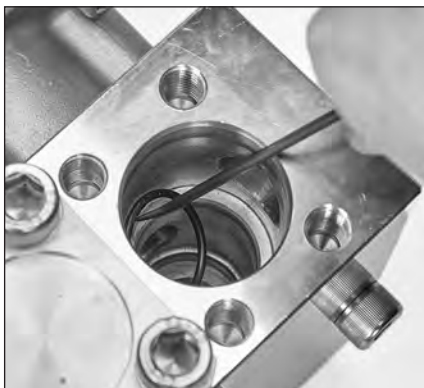
2.07 The valve seat O-ring may remain in the manifold. Use a pick or small flat tip screwdriver to remove O-ring.
