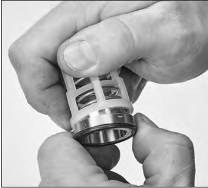
2.18 Remove inlet spring retainer by hand.
