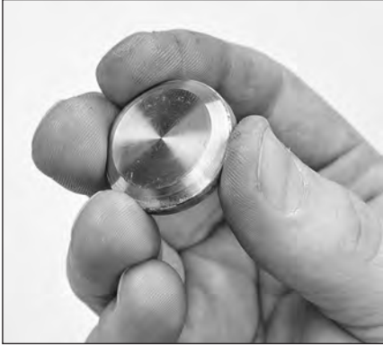
2.21 Inspect tapered surface of inlet valve for wear, pitting or damage.
