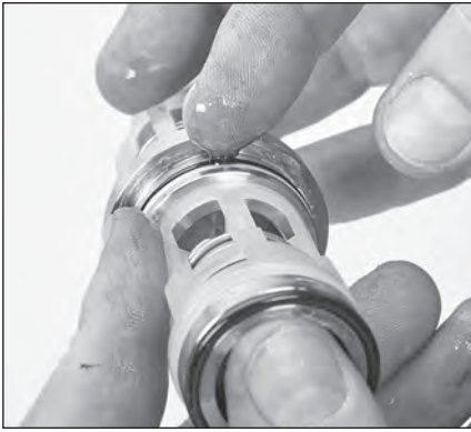
2.37 Apply a lubricant to the outside surface of the discharge valve seat O-ring.
