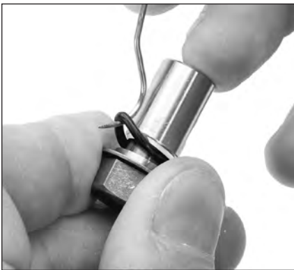
1.26 Using a pick, remove the plunger retainer O-ring from plunger retainer.
