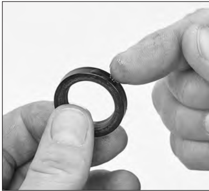
1.39 Apply a lubricant to the outside surface of the low-pressure seals.
