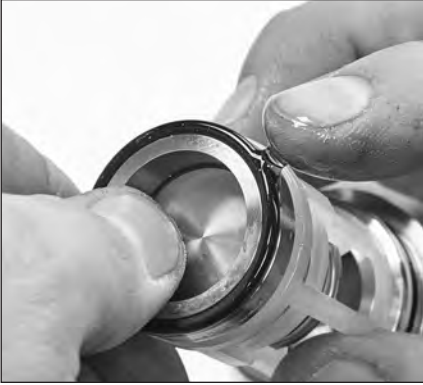
2.36 Apply a lubricant to the outside surface of the inlet valve seat O-ring.
