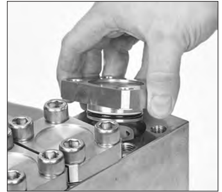
2.03 Remove the valve plug by hand.
