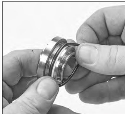
2.30 Replace discharge valve backup ring, then O-ring onto discharge valve seat.
