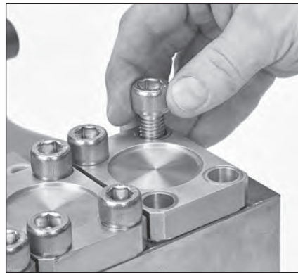
2.41 Install four (4) HSH screws by hand.
