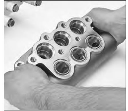
1.41 Flip inlet manifold over so that valve spacer bores are facing up.
